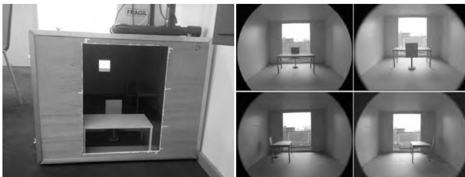
Fig. 2. Scale model and photographs for Back and Front layout (upper), Left and Right layout (lower), with light surfaces
