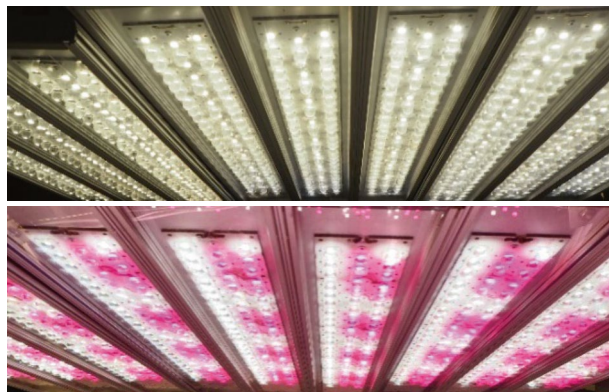
Fig. 1. Appearance of the radiators used for the experiments: ACC-300 (top photo) and ACC-300 Agro (refer to the description in the text)
