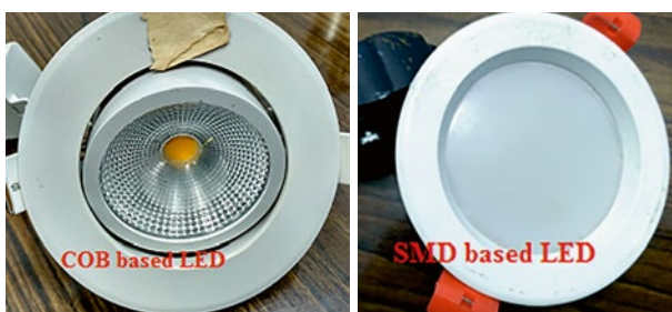
Fig. 1. The selected LED luminaires with external drivers
