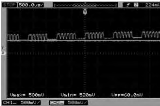
Fig.6a. Time-domain waveform of the OPT101-2 signal
