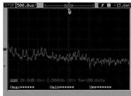
Fig.10b. Spectrum of the input signal
