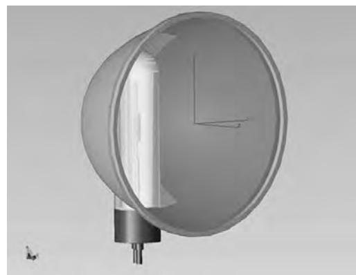
Fig. 5. Model of the luminaire used in the ray tracing simulations
