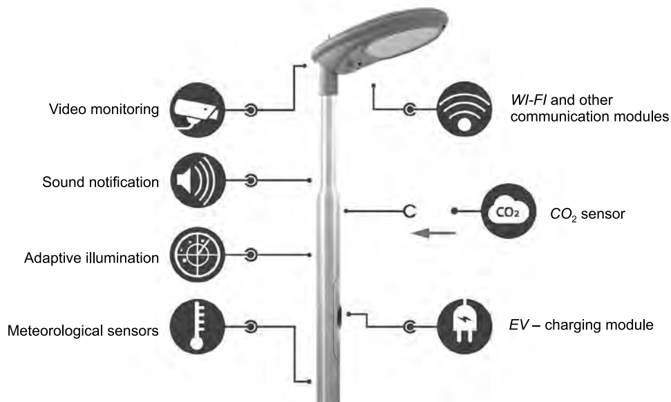
Fig. 18. Schematic image of a street LED luminaire
