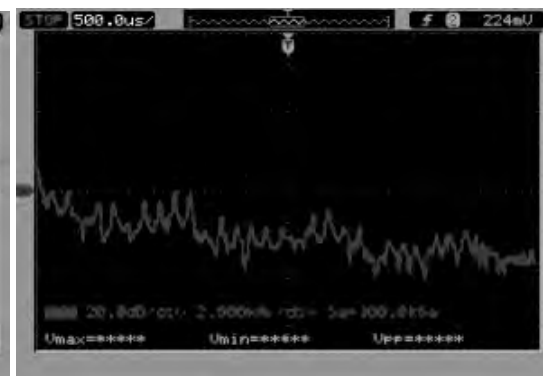
Fig.9b. Spectrum of the voltage comparator signal
