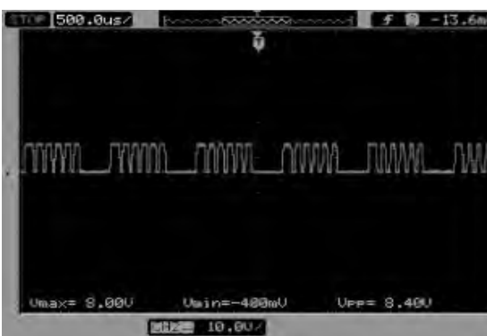
Fig.9a. Time-domain waveform of the voltage comparator signal
