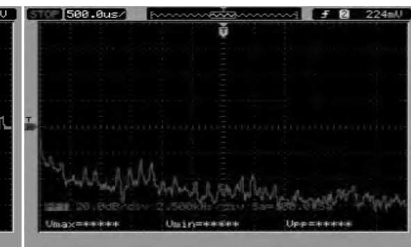
Fig.7b. Spectrum of the difference amplifier signal
