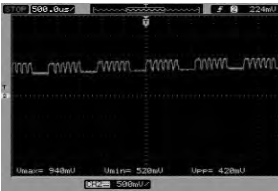
Fig.5a. Time-domain waveform of the OPT101-1 signal
