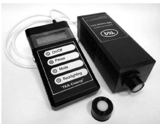
Fig. 1. Appearance of the TKA-SPECTRUM Spectrophotometer device (PAR)
