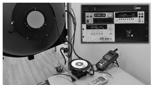
Fig. 2. Temperature controlled Ulbricht Sphere and equipment
