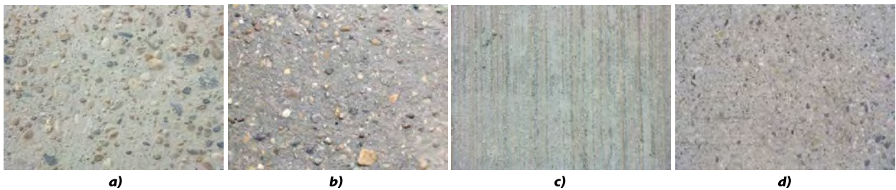
Fig.6. Pictures of the water jet scrubbed concrete (a. initial state, b. after two years); pictures of the broomed surface (c. initial state, d. after 2 years)
