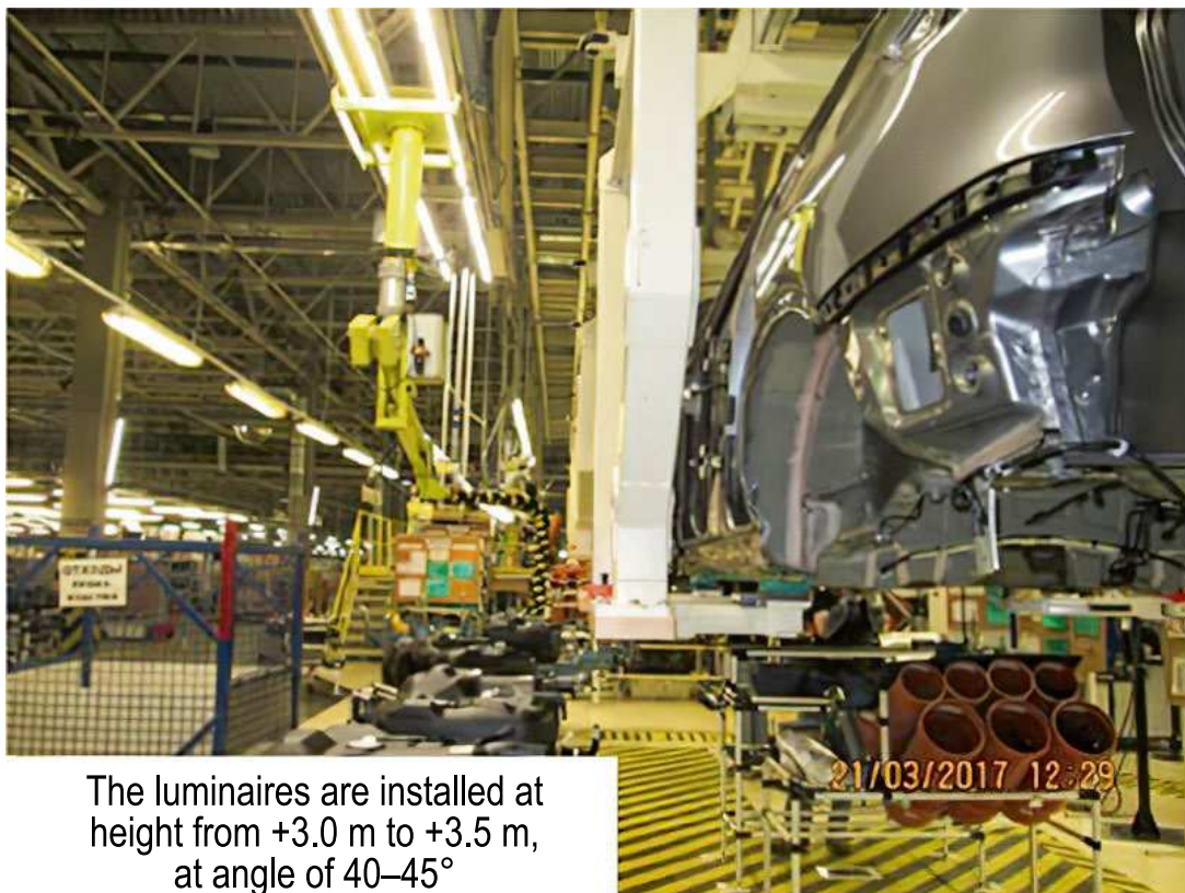
Fig. 2. Active LI of the assembly line
