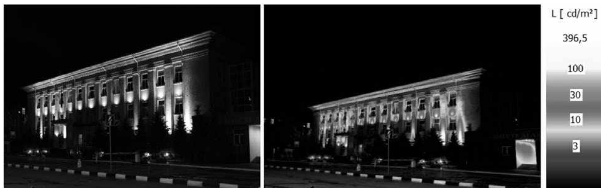
Fig.7. Evening photograph and luminance distribution over the facade, Staronikitskaya st. 1
