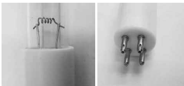
Fig. 6. The exterior of the electrode and the cap
