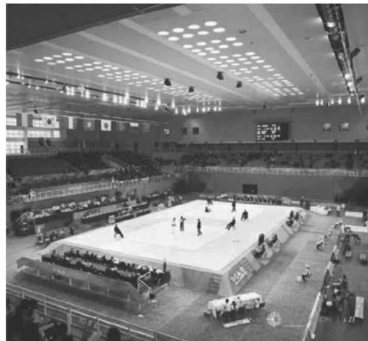
Fig. 10. Illumination of the sports hall of the Peking University using *Solatube*® systems.
