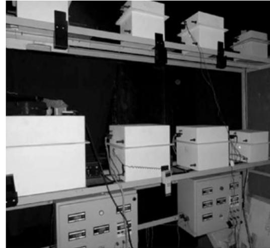
Fig. 2. LED life test rack
