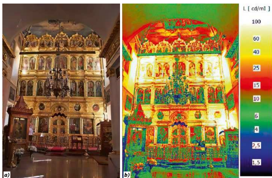
Fig. 9. Lighting of the iconostasis of the Church of St. Nicholas in Tolmachi: Photograph (a) and pseudo-colour luminance distribution (b)
