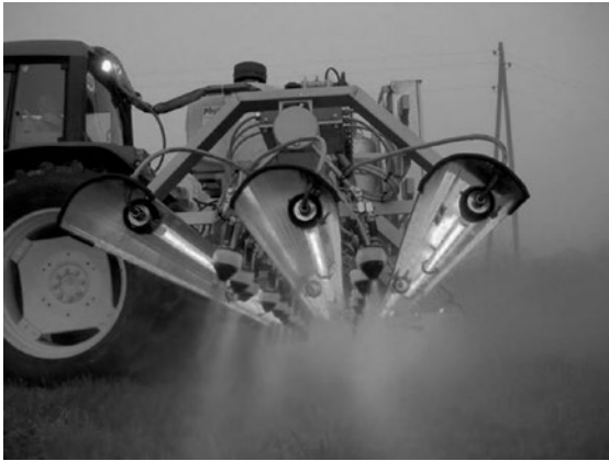
Fig. 7. Platform with UV lamps hung on tractors
