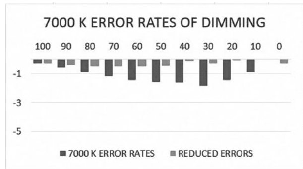
Fig. 16. CCT 7000 K difference rates in dependence of dimming
