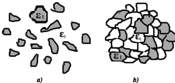
Fig. 1. Topology of composites: (a) cermets: discrete impregnations into a matrix (b); aggregates: symmetric filling of a composite without selected matrix [23]
