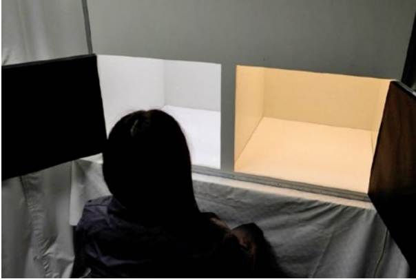
Fig. 1. The subject compared the brightness of the two chambers when the luminance of the two chambers was the same, i.e. at equi-luminance, either at 267.6 \text{ cd/m}^2 or at 24.8 \text{ cd/m}^2 ; here, the reference stimulus appears on the left (“2 nd series”)
