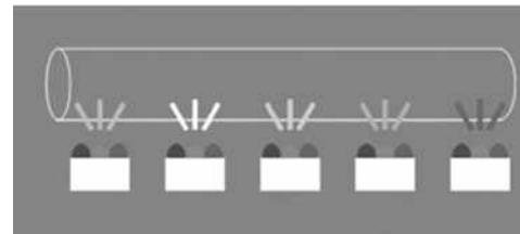
Fig. 3. Colour lighting of motor car interior with mono-chrome or polychrome LED’s with application of a light guide and a colour adjusting device
