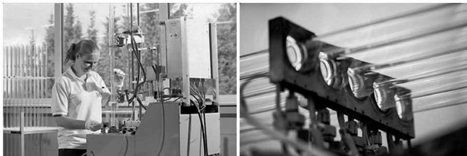
Fig. 8. Production of amalgam lamps
