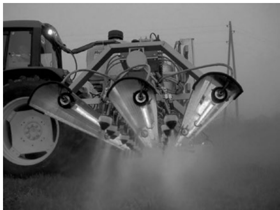
Fig. 7. Platform with UV lamps hung on tractors
