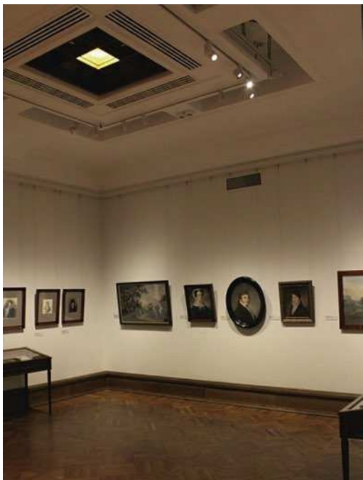
Fig. 3. Hall of Graphics. Illuminance of exhibited items at a height of 1.6 m due to accent lighting is 60 lx
