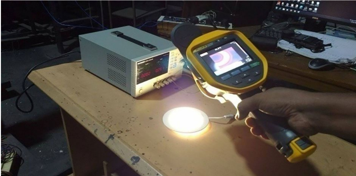
Fig. 1. Temperature measurement of the LED without driver by using Thermal Imager (Fluke Ti 400) methodology adopted
