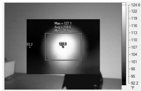
Fig. 3. Thermal image of COB type warm white LED after 60 min burning
