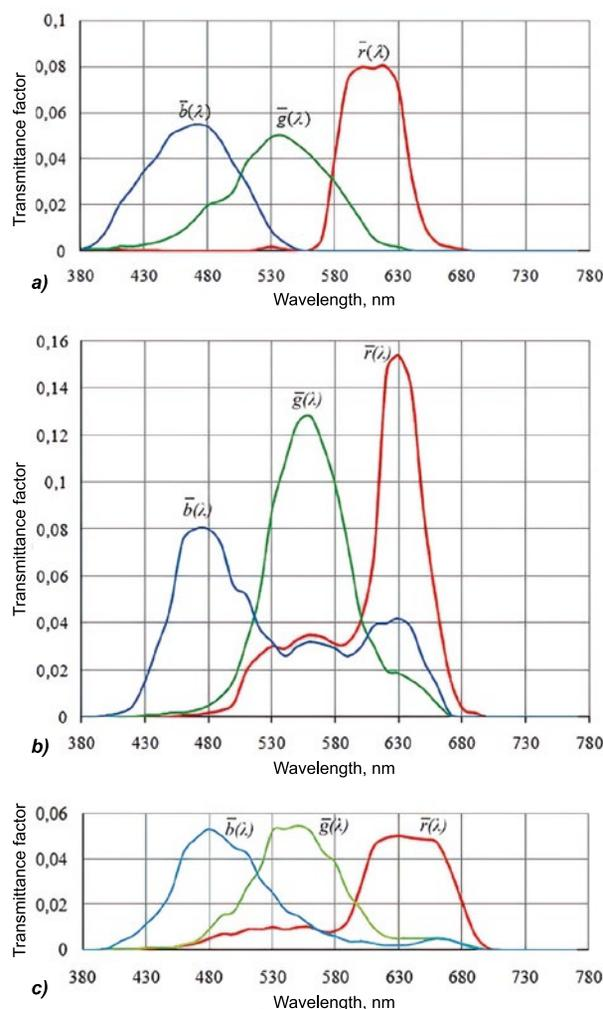
Fig. 1. Spectral characteristics of matrix photo detectors *Sony* (a), *Kodak* (b) and *Agilent* (c)
