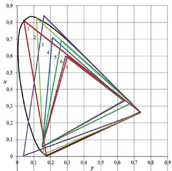
Fig. 2. The studied colour spaces on the  $x, y$  colour space: 1 – *MINIPI*; 2 – *Wide Gamut RGB*; 3 – *ProPhoto RGB*; 4 – *AdobeRGB*; 5 – *DCI-P3 RGB*; 6 – *PAL/SECAM*; 7 – *sRGB*
