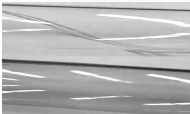
Fig. 3. Quartz walls of a new lamp envelope (above) and of an exhausted lamp envelope
