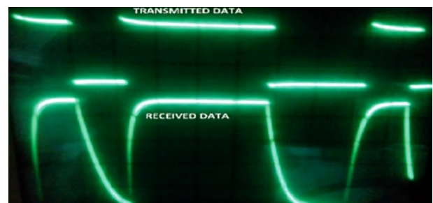
Fig. 14. Measured transmitted and received bit pattern (in presence of daylight)
