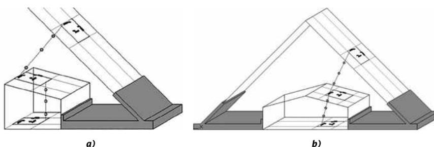
Fig. 13. Scheme of positioning of temperature and heat current sensors:
