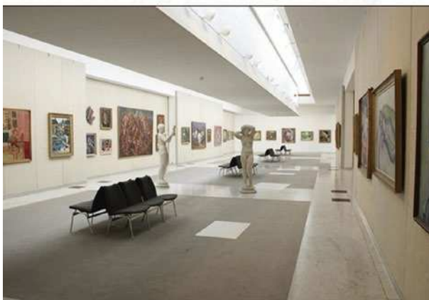
Fig. 10. Museum of Art in Alborg, Denmark (A. Aalto, 1958–1972). Transformation of direct sunlight into diffused light by means of lanterns of complex shape. Section and view of the day interior
