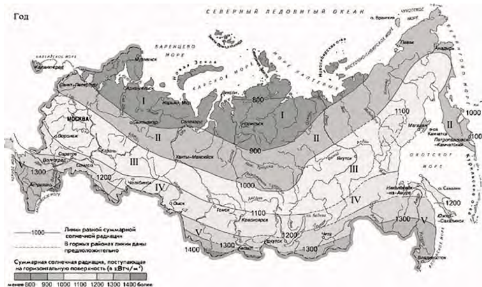
Fig. 4. Schematic map of total annual solar radiation on a horizontal surface in conditions of actual cloudiness, kWh / m^2
