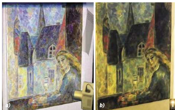
Fig. 8. Comparison of a painting with optimal lighting by means of a controllable LS with T_{cc} = 5000 K (a) and of an incandescent lamp with T_c = 2800 K (b)
