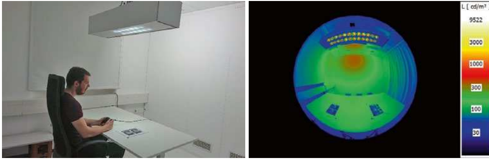
Fig. 4. Experimental setup used for the second experiment for directional lighting, locally increasing the illuminance level on the office desk, was realized by a custom-made test luminaire enabling the adjustment of its luminous intensity distribution (ambient illumination was provided by a soft-light LED panel, which was hidden behind the suspended test luminaire and pointed towards the white opposing wall defining the luminance distribution in the observers' peripheral field of view): (a) with the help of an Xbox 360 controller, participants were able to adjust the local dimming of the illumination of the office desk according to their preference for task performance; (b) reference condition of homogeneous desk illumination
