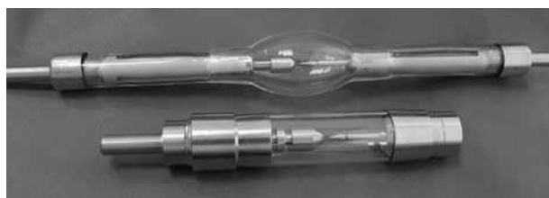
Fig. 1. Design of UHP xenon lamps with quartz ball envelope and cylindrical sapphire envelope
