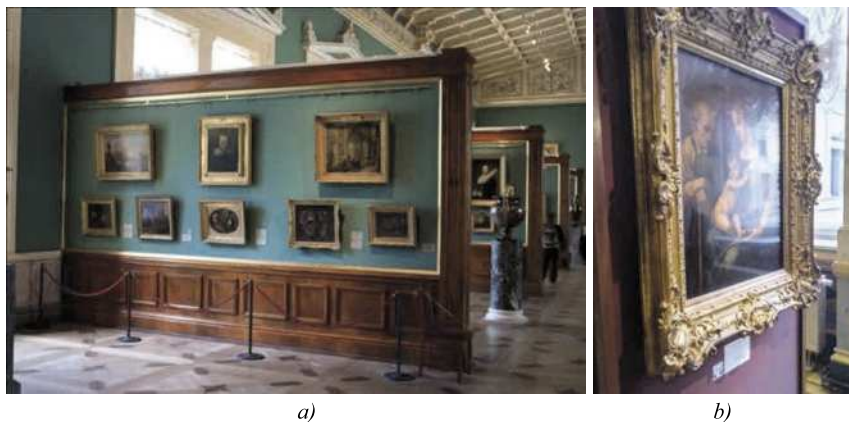
Fig. 8. Glare on paintings located perpendicular to a window: a) without protective glass; b) with protective glass
