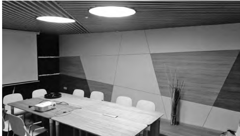
Fig.8. Meeting Room (Daylight illuminance about 400 lx at high clouds of the sky. In sunny weather, natural light flow is regulated by means of dimmer, which allow to regulate the natural light flow and to perform a complete shutdown of natural lighting during video presentations)
