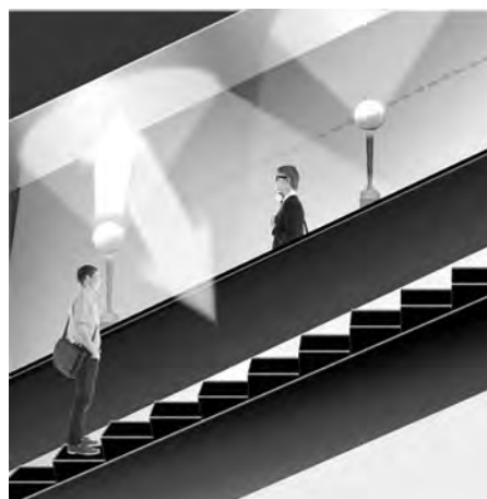
Fig. 5. A proposed illumination layout of an escalator: visualisation of escalator inclination illumination principle
