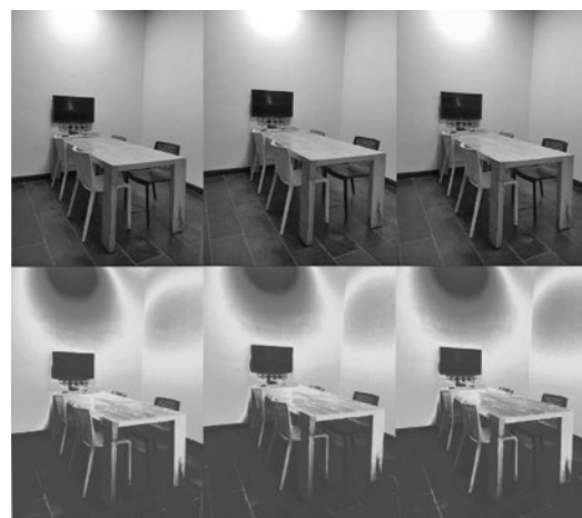
Fig.1. Experimental room with tuneable LED lighting system generating three scenes of CCTs 3000 K, 4000 K and 6500 K respectively at an average constant illuminance of 300 lx at the table-top
