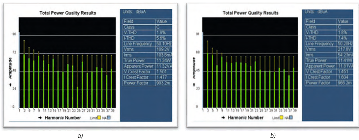
Fig.7. Harmonic testing results: (a) 110Vac Input; (b) 220Vac Input
