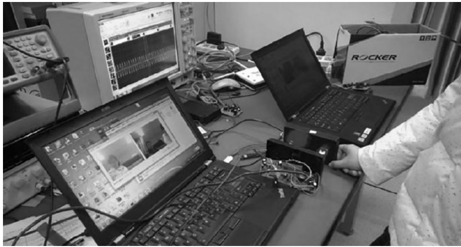
Fig.2. Two computers are connected by visible light module
