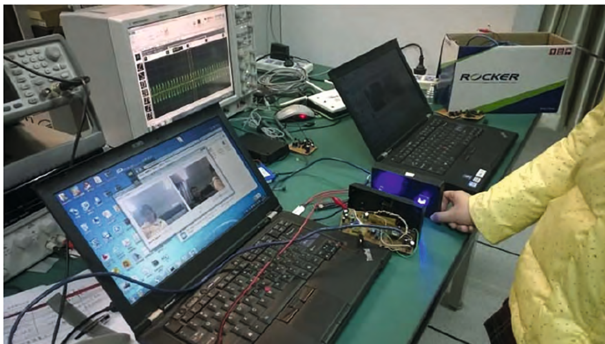
Fig.2. Two computers are connected by visible light module
