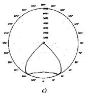
Fig. 1. Diora Craft 110/13000 luminaire (capacity of 110 W, luminous flux of 13,000 lm,  $T_{cp}$ =5000K, *IP65*): *a* and *b* – general view of the luminaire; c – LDC
