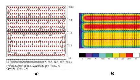
Fig. 3. Design fragments of the project of lighting of production areas of building No. 4. Design distribution of illuminance in iso-illuminance curves (*a*) and fictitious colours (*b*)
