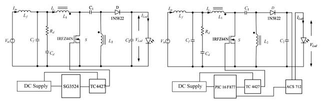
Fig. 11. Application circuit of SEPIC converter
