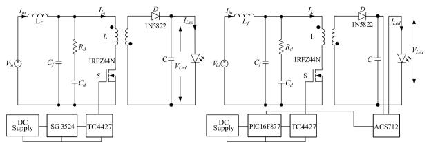
Fig. 13. Application circuit FLYBACK converter
