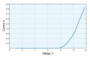
Fig. 1. Voltage-current characteristic of power LED
