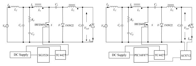
Fig. 12. Application circuit CUK converter
