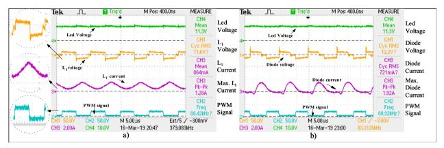
Fig. 15. SEPIC converter: a – LED voltage ( $V_{LED}$ ), input side inductor voltage ( $V_{LI}$ ) and current ( $I_{LI}$ ), PWM signal; b – SEPIC converter input voltage ( $V_{in}$ ), diode voltage and current, PWM signal
