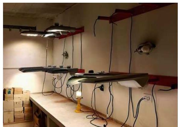
Fig. 5. Aspects of 6,000 h operation test (photo from author)
