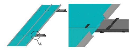
Fig. 9. Fixation of the lantern light glaring elements to horizontal guides
