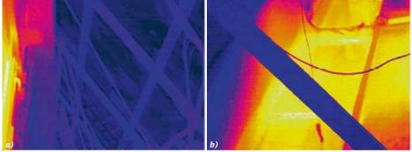
The thermal imaging inspection of the examined structure was performed at ambient temperature of  $t_a$ = -4.5 °C and internal air temperature of  $t_i$  = +20 °C (Fig. 12).
