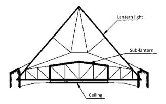
Fig. 5. Cross-section of the transparent structure
